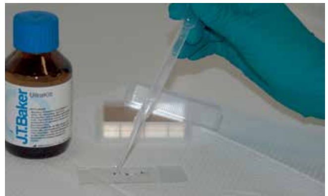
Fig.7 Drops of UltraKitt™ mounting media should be placed on the slide
